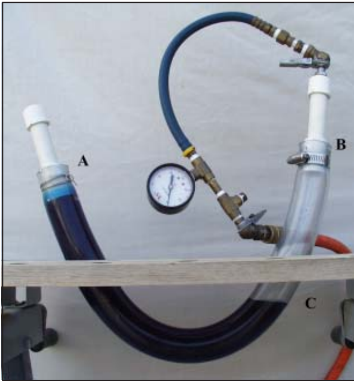
Figure 3 The test setup, at full pressure, on the ClampTite clamp.
