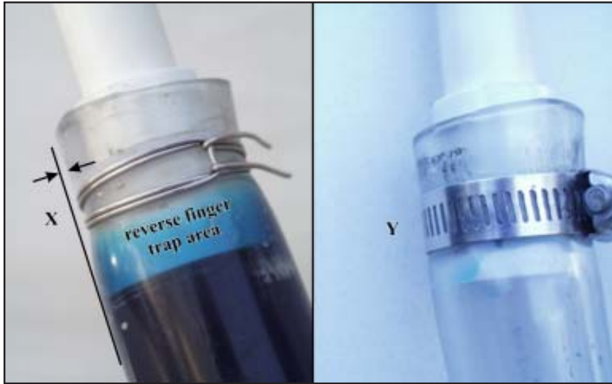
Figure 5 Clamp indentation is a sign of holding force.
