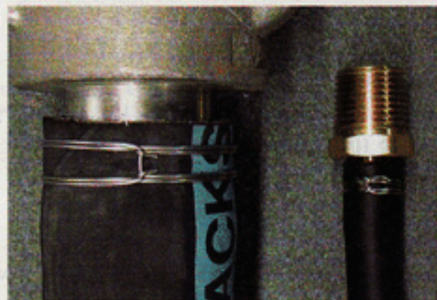
The writer used the tool to clamp several sizes of hose, including a 1-1/2-inch exhaust hose and a 3/8-inch SAE fuel line.
